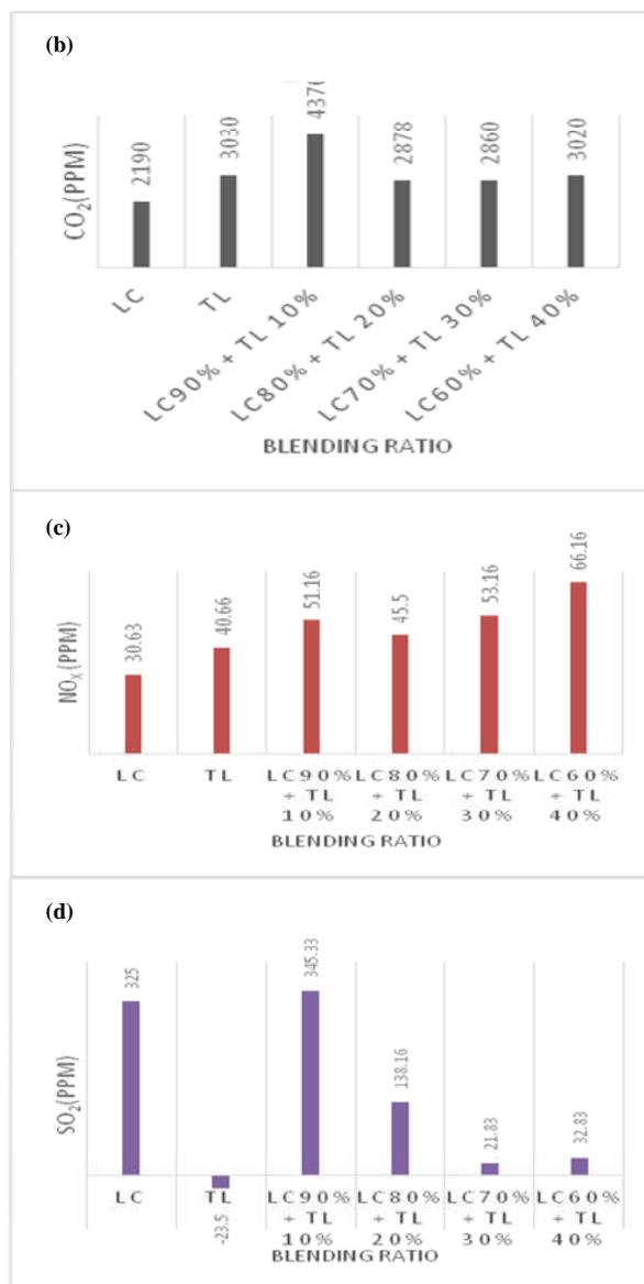
Figure 4. Effect of different blending ratio of coal and tree leaves on (a) CO, (b) CO<sub>2</sub>, (c) NO<sub>x</sub> and (d) SO<sub>2</sub>
