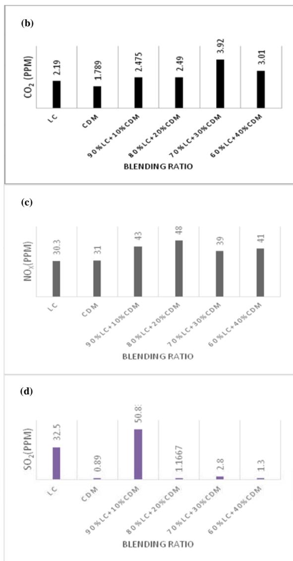
Figure 2. Effect of different blending ratio of coal and cow dung manure on (a) CO, (b) CO<sub>2</sub>, (c) NO<sub>x</sub> and (d) SO<sub>2</sub>
