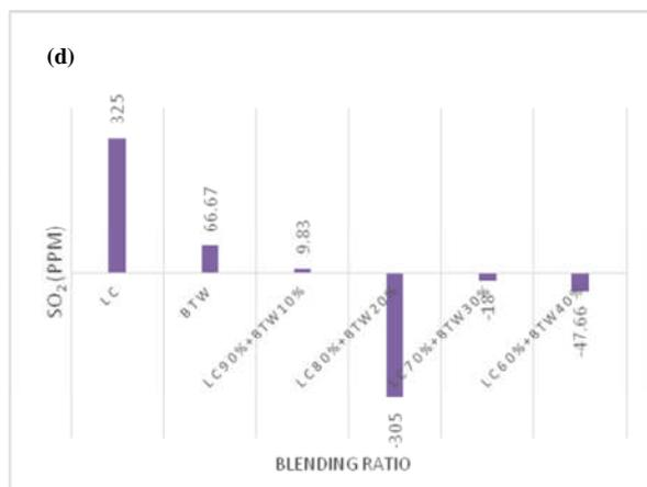
Figure 3. Effect of different blending ratio of coal and banana tree waste on (a) CO, (b) CO<sub>2</sub>, (c) NO<sub>x</sub> and (d) SO<sub>2</sub>
