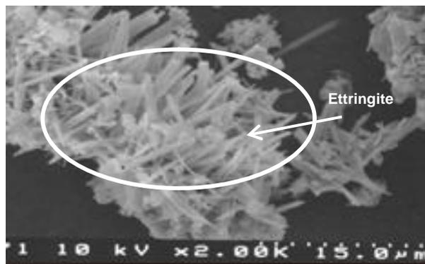
Figure 1. Ettringite observed in the dried products after the coagulation.
