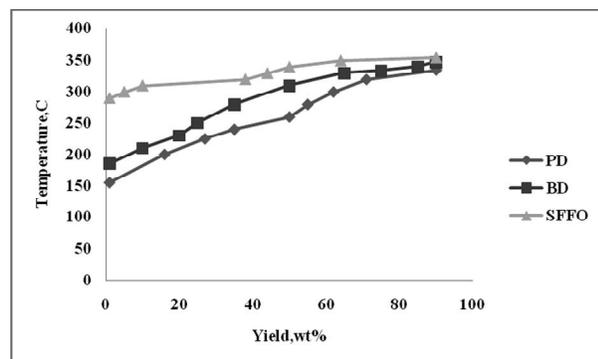
Figure 3. Distillation curves (ASTM D1160) of SFFO and its BD fuel.
