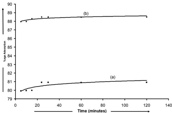
Figure 1. Effect of shaking time on %age Adsorption at (a) 10ppm, (b) 40 ppm for CN<sup>-</sup> adsorption on Alumina.
