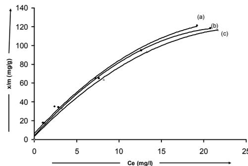
Figure 2. Adsorption isotherms of CN<sup>-</sup> on Alumina at different temperatures: (a) 283K, (b) 313K, (c) 323K.
